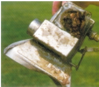
Engine air intake blocked by Belgian racing pigeon. The aircraft was at 500 ft and 140 kts practising for an air race round the Isle of Wight. Aircraft force landed on the beach.
