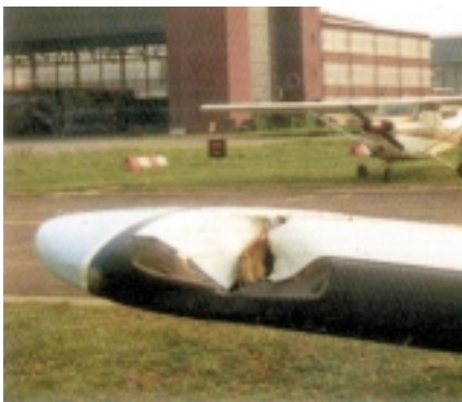
Damaged Piper Aztec wing after collision at 105 kts with a Grey Heron (weight 1.5 kg)
